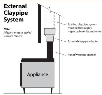
For use where there is sufficient room to "cup" the end of the clay liner
