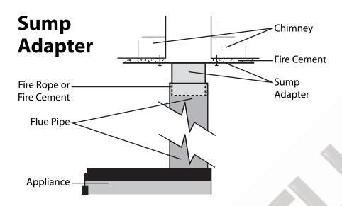
The sump adapter is inserted into the bottom of the flue pipe and then fixed to the chimney. It is sealed with Fire Cement or Fire Rope where the Sump Adapter sits in the flue pipe.
