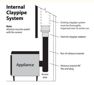
For use where there is limited room and you can only insert up into the clay pot.
